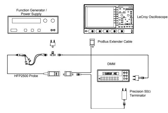
Figure 7-2. Offset and LF Attenuation Accuracy Test Setup
