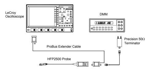
Figure 7-1. Output Zero Voltage Test Setup
