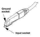
The small, low mass probe head is designed for ease of use and high performance.
