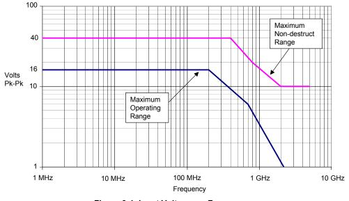
Figure 9-1. Input Voltage vs. Frequency
