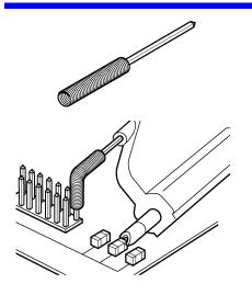
A flexible spring connected to a square pin that fits into either of the probe sockets. Designed to be attached to a square pin on the circuit under test.
