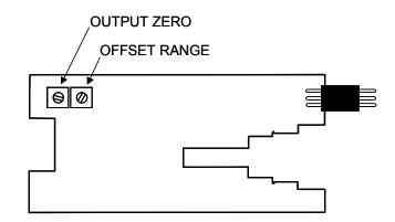
Figure 8-2a. Adjustment Locations S/N 1000 and higher
