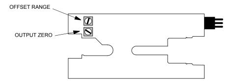
Figure 8-2b. Adjustment Locations S/N below 1000.
