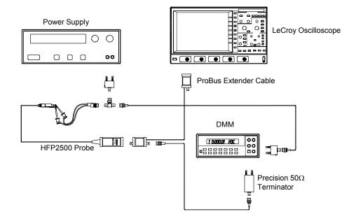
Figure 8-3. Offset Range Adjustment setup.
