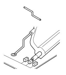
The offset pin is designed to be attached to either socket of the probe head. The offset pin is the highest quality grounding solution and is recommended in high frequency applications.
