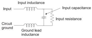
Figure 5-1. Probe Input Equivalent Circuit
