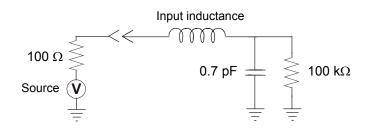
Figure 5-2. Probe input equivalent circuit
