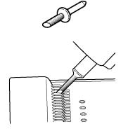
The straight tip is rugged and designed for general probing. Fits in either probe socket.
